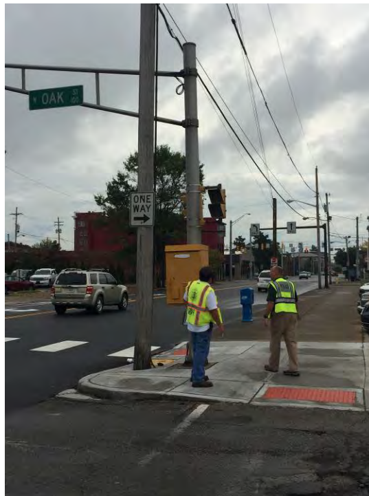
Photo 13: RSA audit of an intersection where crosswalk markings are still needed at one approach.
