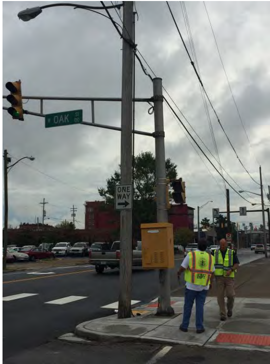
Photo 14: Several poles on a corner are a reminder to consolidate projections when possible.
